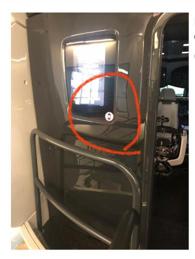
If the ramp does not operate following selection of "MOTION OFF" use ramp controls on left rear exterior and select arrow down
